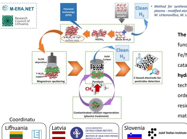
Method for synthesis of gamma aluminium oxide using plasma - modified aluminium and water reaction. D. Milčius, M. Urbonavičius, M. Lelis. EPO, EP3768640B1
