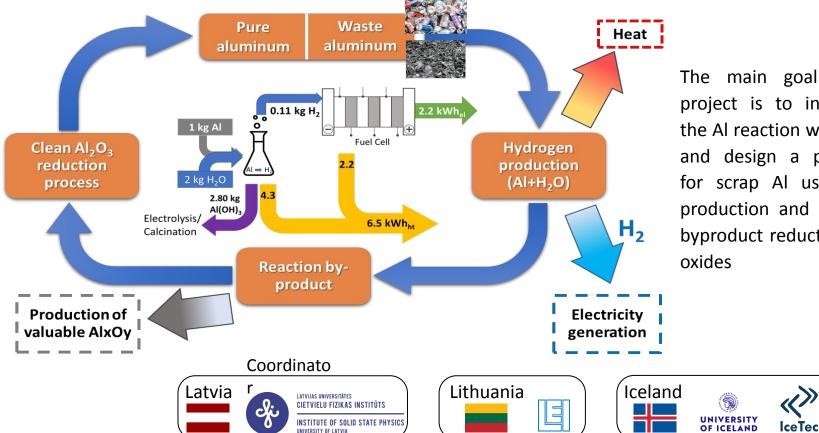
The main goal of the project is to investigate the Al reaction with water and design a prototype for scrap Al use in H<sub>2</sub> production and following byproduct reduction to Al
