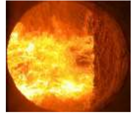
NH 3 / pulverized coal flame
